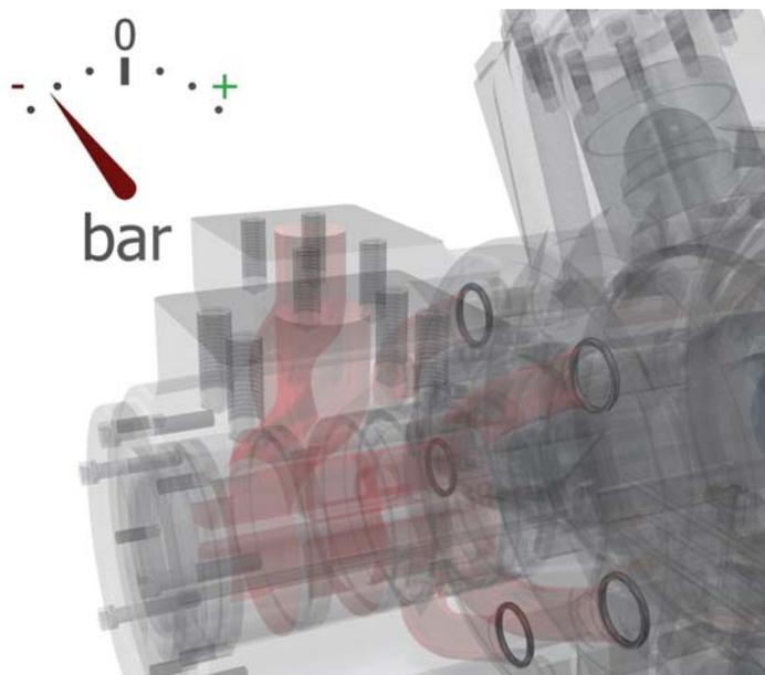
Cavitation can occur due to many different factors. Although it is not possible to make the HMB motor resistant to cavitation, certain features can be added to improve the motor's resistance to short periods of lost port pressure.
